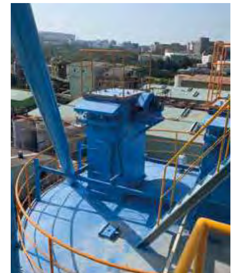
Goldsun works to prevent air pollution. Our dust collectors minimize dust pollution during processes.
